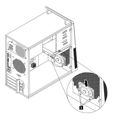
Figure 47. Installing a new internal speaker
